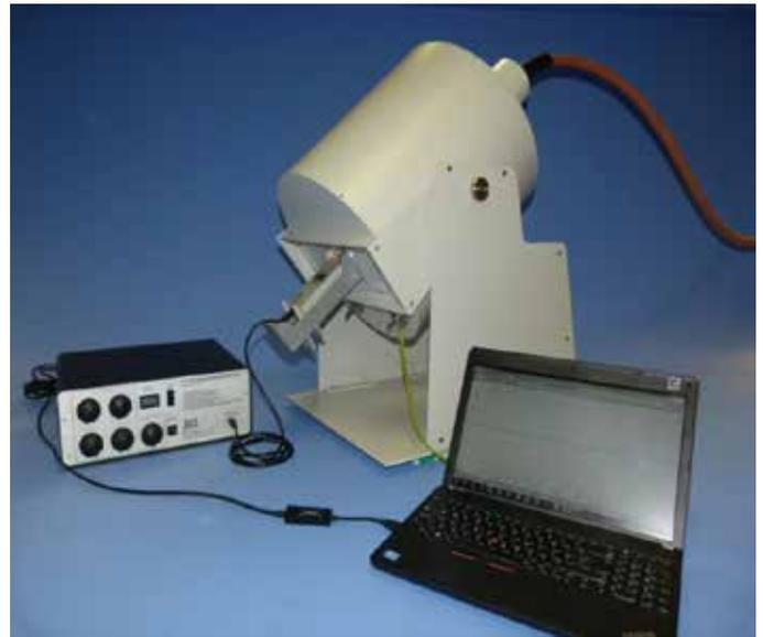
JCI 146 voltmeter adapter shown with JCI 140 static monitor and optional JCI 165 optoisolated USB data acquisition module and laptop (laptop not included)
